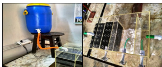
Figure 7: Equalization tank connected with Reactor Figure 8 : Flexural plastic PVC pipe adjust with dispenser water tap
