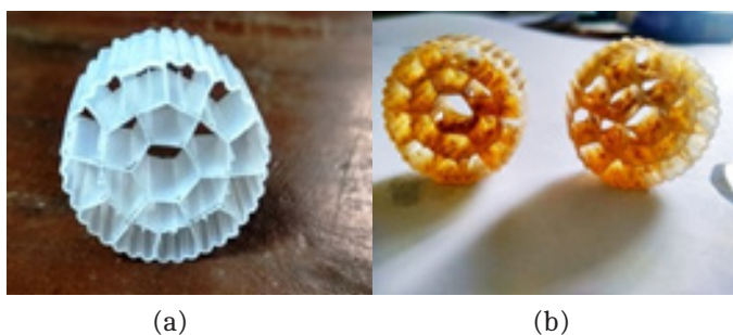
Figure 16: (a) kaldnes K3 media before using in experiment (b) kaldnes K3 media after ending the experiment with biomass
