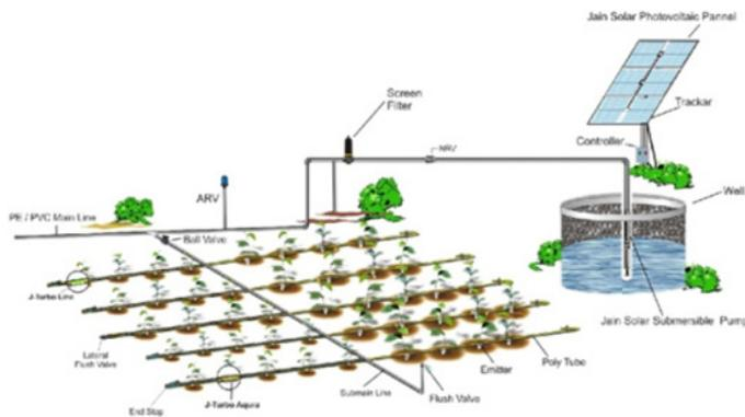
**Figure 1:** Showing the schematic design of Solar Drip Irrigation. to ruin the field of Agriculture crops.
